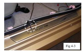
(c) Clean the pinch weld surface behind the door sill harness with a wiping cloth and a VDC approved cleaner. (Fig. 4-3)
